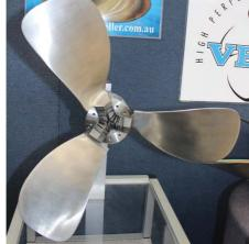
top: Electrolysis can be a major risk for saildrives so beware when you fit a new folding propeller in terms of the metal mix. *Photo Kevin Green* above: The stainless Austral Slipstream folding propeller fits shaft and saildrives from 12-20 inches on all major engine manufacturers. It's available in two or three blades. *Photo Kevin Green*
