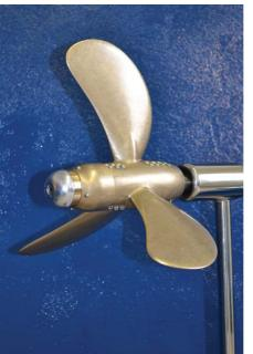
The Italian Marine made J-Prop range is supplied by Calibra Marine UK and offers mechanical pitch adjustment for their models that are 2-blade, 3-blade and 4-blade propellers for 8hp to 400hp engines; in both shaft and sail drives. Photo Calibra Marine (UK)
