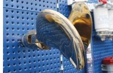
Volvo range of folding propellers comprise 2, 3 and 4-blade models for both shaft and saildrives; and of course are built specifically for their engine gear ratios for maximise performance. Photo Kevin Green
