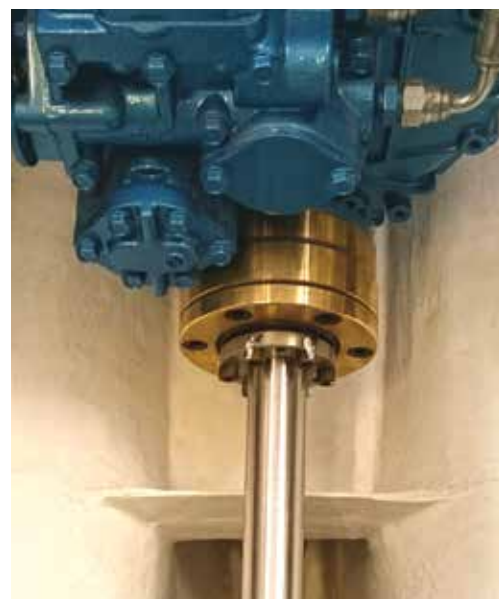
When repowering, it makes sense to upgrade the rest of your drivetrain as well: (above) a Vetus shaft coupling and muffler; (below) a SigmaDrive coupling from Bruntons
